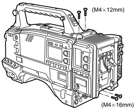
4 Connect the connectors on the battery mount to the connectors on the camera adapter.
