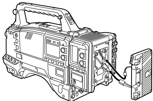
5 Use the screws to screw the battery mount onto the camera adapter.
